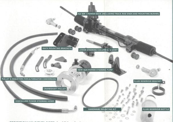
**SPECIFICALLY DEVELOPED** for Mk2 enthusiasts, our new power rack and pinion steering kit is the most comprehensive of its kind.
