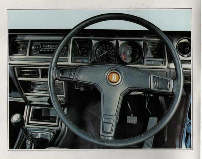
Light-touch recirculating ball steering requires less effort to operate and gives you a small turning radius so that parking is much simpler. Dual-circuit brakes have a powerful servo so that you can stop safely and swiftly with the minimum of effort, while a slick 4-speed, all synchromesh gearbox and a light clutch add to the all-round ease of driving.
