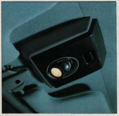
A roof mounted console incorporates a useful swivel map reading light.
