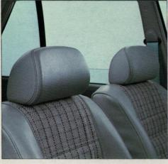
Front seats on the New Bluebirds are fitted with adjustable head restraints.
