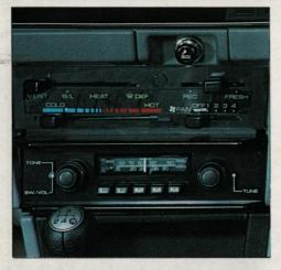
An impressive centre console houses controls for the advanced heating and ventilation system, a pushbutton radio and cigar lighter.
