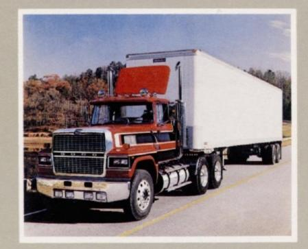
The functional aerodynamic design of the LTL hood also permits downward sight lines . . . as good as the shorter hood LT-Series.
