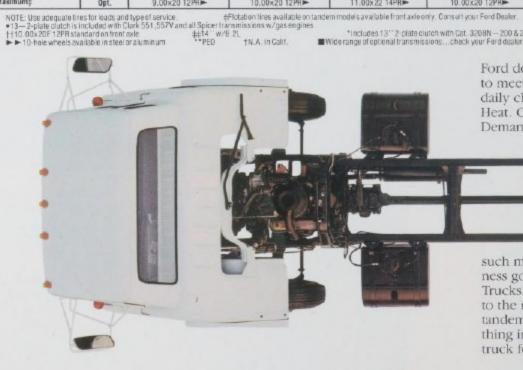
Ford tilts its entire cab for easy access. The C-Series cab easily tilts 45° exposing the engine, clutch, transmission and accessories for convenient routine service or repairs.
