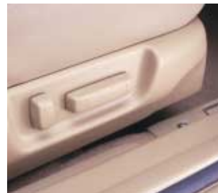
Executive models feature electric driver seat controls, with effortless eight-way adjustment including 40mm of height and 80mm fore-and-aft.
