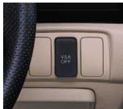
The Vehicle Stability Assist (VSA) system fitted as standard on 2.4-litre models.
