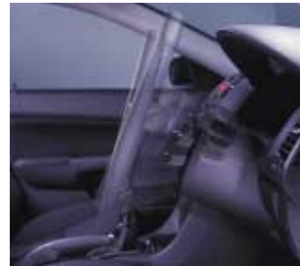
Four degrees of tilt adjustment ensures maximum comfort and a clear view of the instruments.
