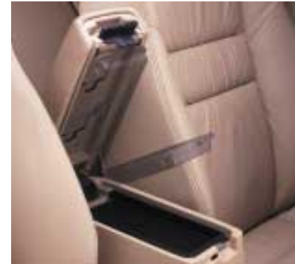
The armrest lifts to reveal a shallow trinket tray, which can be raised using a separate lever to open up the deeper storage box underneath.
