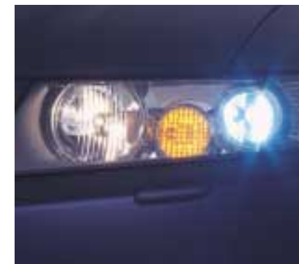
New projector-style headlamps improve visibility and safety, with powerful high-intensity gas discharge (HID) headlamps which are standard on the 2.4 Executive model.
