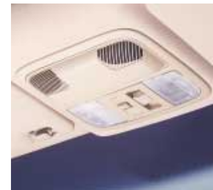
On Executive and Type S models the ultrasonic alarm is discreetly stored in place of the sunglasses holder, for optimum interior monitoring.
