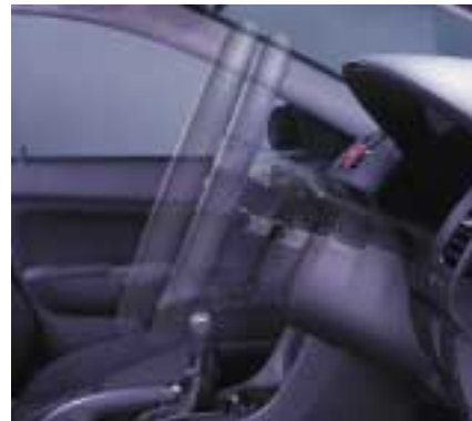
The steering wheel has 40mm of telescopic adjustment to give you the perfect reach.
