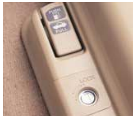
With its interior release mechanism, the boot opens by pulling the lever located next to the driver's seat. A gentle touch of the lever opens the fuel filler flap, which can be locked from inside the car.
