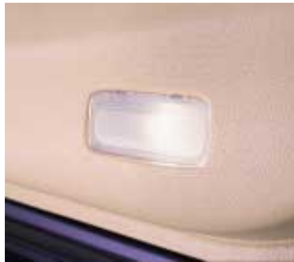
A warning light illuminates automatically as soon as either front door is opened.
