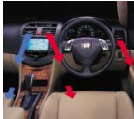
The dual zone climate control allows front seat passengers to set temperature independently.
