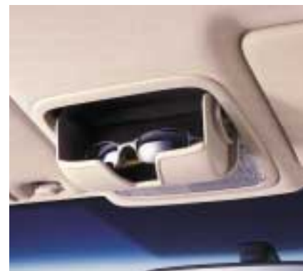
The sunglasses holder is conveniently located directly above the driving mirror and fitted with a secure damped-action cover on SE and Sport models.
