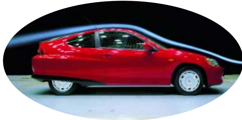
35% increase in fuel efficiency through weight reduction measures and advanced aerodynamics
