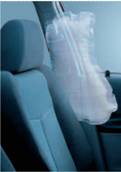
All round impact protection is ensured by the presence of driver, passenger and side airbags.
