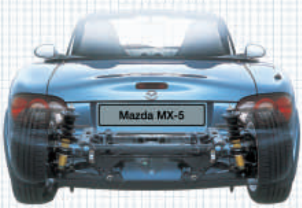
Superb handling, whichever way you look at it. Coupled with an ultra-stiff chassis, the Mazda MX-5 features classic double-wishbone suspension all round.
