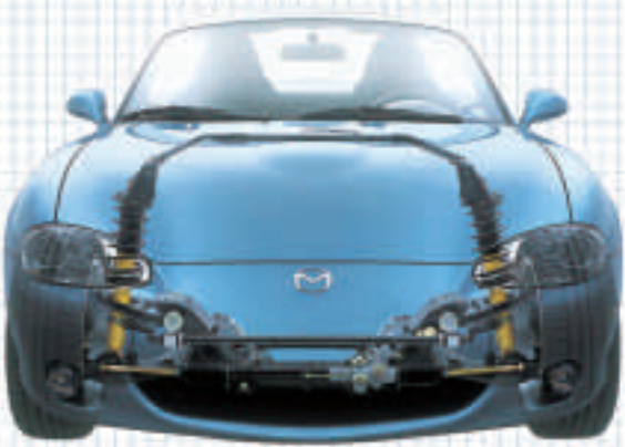
Superb handling, whichever way you look at it. Coupled with an ultra-stiff chassis, the Mazda MX-5 features classic double-wishbone suspension all round.
