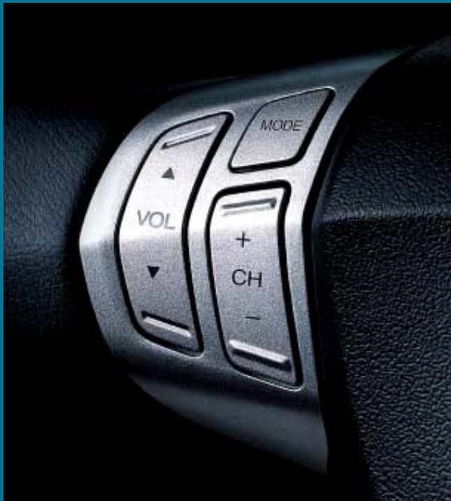
The remote audio controls are mounted on the steering wheel for greater convenience and safety.
