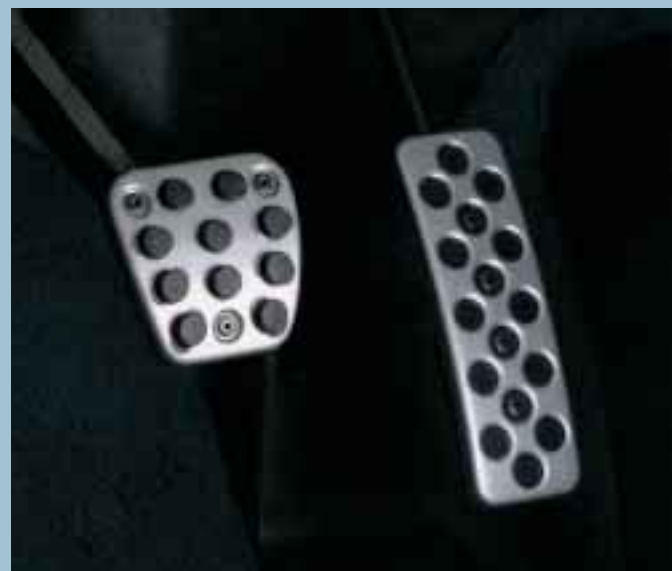
The foot pedals are drilled aluminium alloy making them light and sensitive for instant, precise responses.
