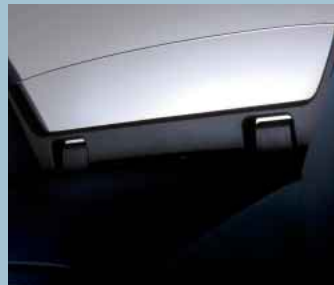
Turbulence in the cabin is reduced, thanks to the folding wind deflector, located between the rear headrests.
