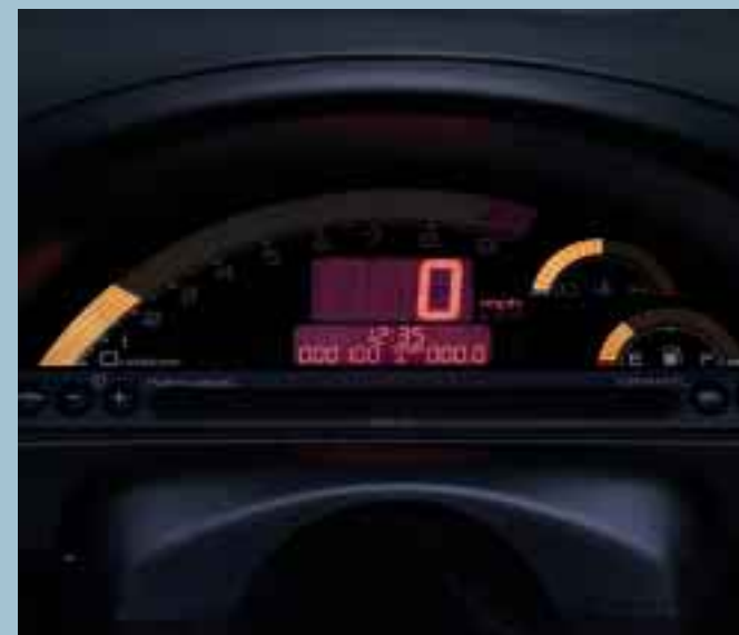
The Honda S2000's instrument panel is an easy to read digital display.
