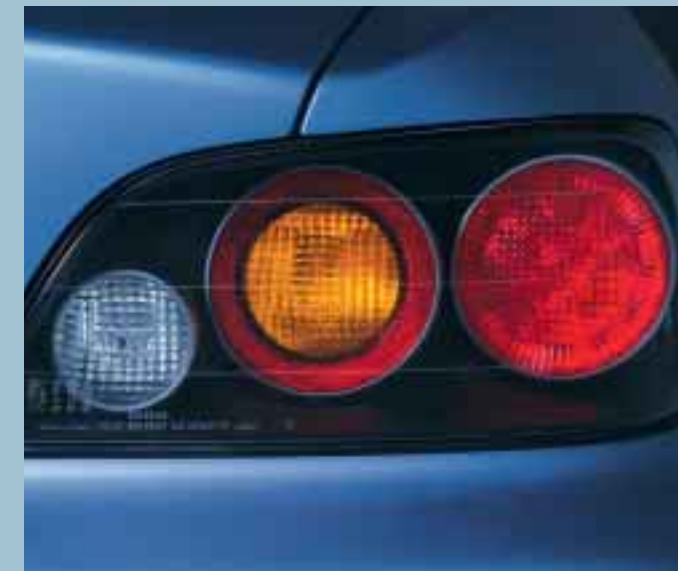
High intensity LED rear brake lights sit with the reversing and driving lights behind impact resistant aerodynamic covers.
