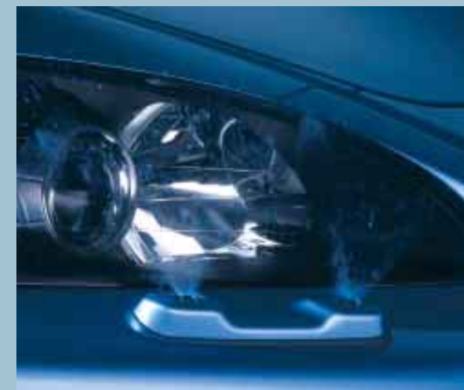
To ensure that the HID headlamps maintain their efficiency, powerful headlight washers are fitted as standard.
