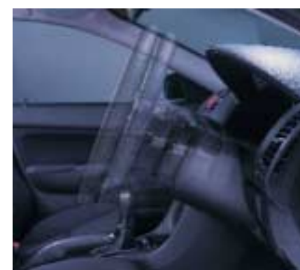
The steering wheel has 40mm of telescopic adjustment to give you the perfect reach. Four degrees of tilt adjustment ensures maximum comfort and a clear view of the instruments.
