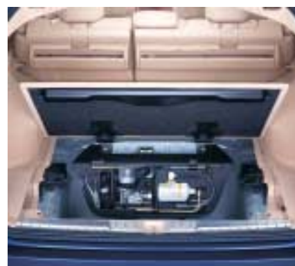
Instead of carrying around a heavy spare wheel, the Accord Tourer is equipped with a tyre repair kit, consisting of repair fluid and an air compressor powered by the car's 12V outlet. (Space saver spare wheel is available as an option.)
