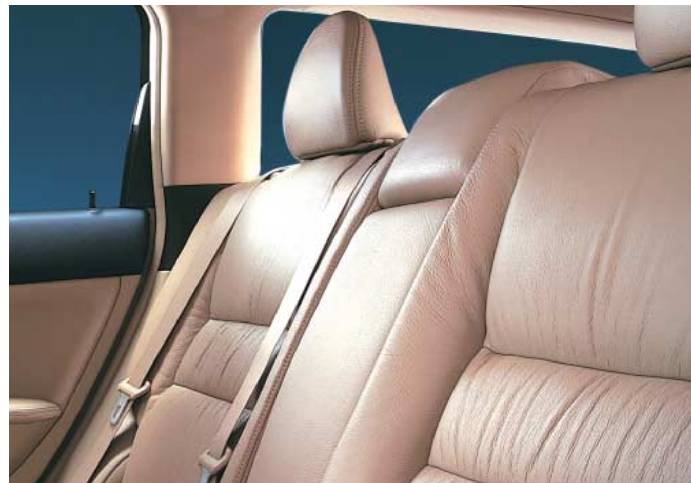
The three rear head restraints and three-point seatbelts are fully integrated into the seat back as part of the Tourer's unique One Motion rear seat folding mechanism.
