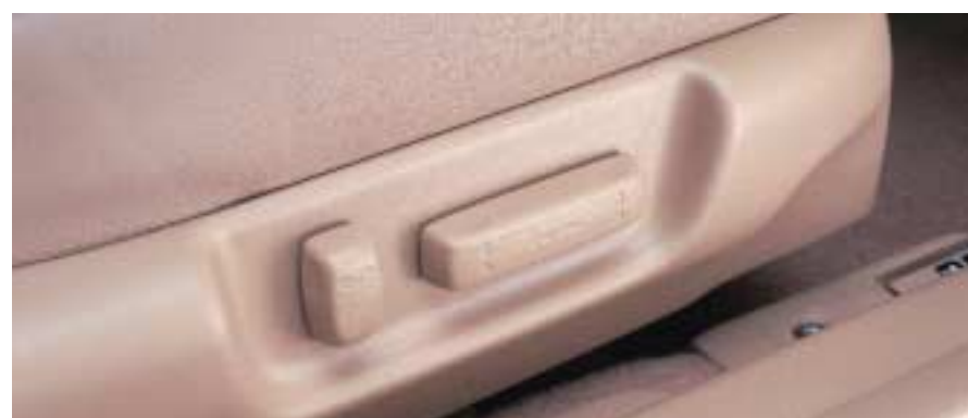
Executive models feature electric driver seat controls, with effortless eight-way adjustment including 40mm of height and 80mm fore-and-aft.
