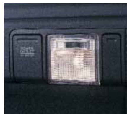
12V power outlet, handy hook and luggage area lights are located on both cargo walls.
