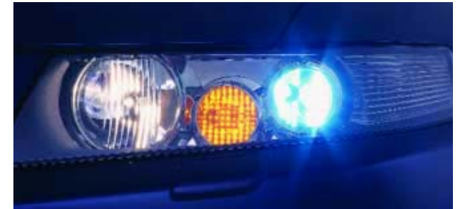
Projector-style headlights improve visibility and safety, with powerful high-intensity gas discharge (HID) headlight which are standard on the 2.4 i-VTEC Executive model.
