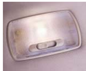
Interior lights come on at full intensity when the doors are unlocked, and remain lit for 30 seconds, before gradually fading out.
