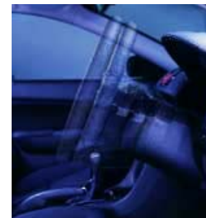
The steering wheel has 40mm of telescopic adjustment to give you the perfect reach. Four degrees of tilt adjustment ensures maximum comfort and a clear view of the instruments.
