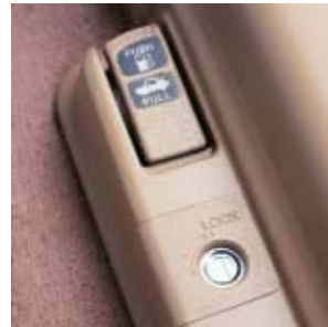
Both the boot and fuel filler cap are opened with a gentle touch of a lever next to the driver's seat. For extra security, the lever can be locked to prevent them being opened from inside the car.
