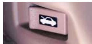
Set into the footwell moulding, the bonnet release lever is unobtrusive yet easily accessible.
