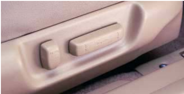
Executive models feature electric driver seat controls, with effortless eight-way adjustment including 40mm of height and 80mm fore-and-aft.
