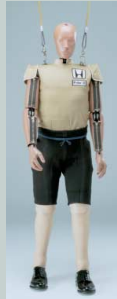
By replicating the human body, our unique POLAR II dummy raises pedestrian safety to outstanding levels.
