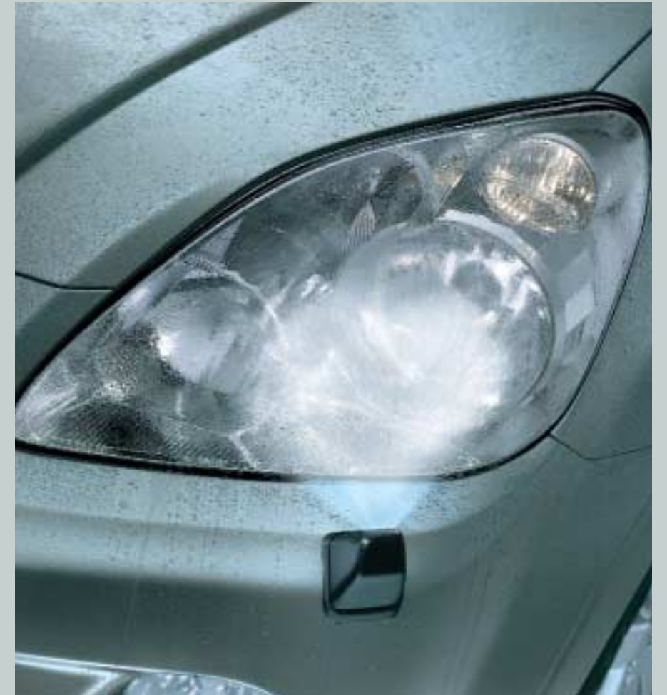
Headlight washers on the Sport and Executive models ensure your lights are always at maximum brightness.
