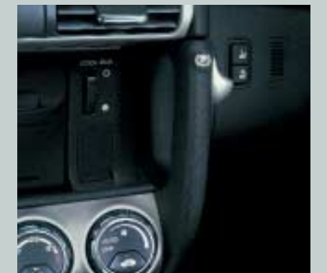
The handbrake is positioned in the dash for ease of use, style and space.
