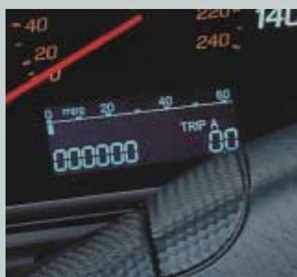
The trip computer tells you how far you have travelled in miles per gallon, plus instantaneous and average fuel consumption.
