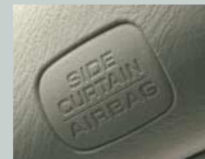
Curtain airbags provide additional protection from side impacts.
