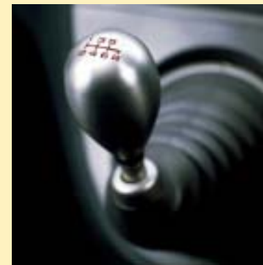
Gearshift - An alloy gearshift connects you to the six speed close-ratio gearbox on the Type-R.
