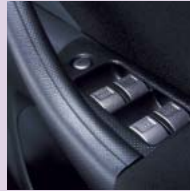
Driver's door panel - All controls for driver and passenger windows are tactile and laid out logically for easy, intuitive operation. Driver control button deactivates all window switches when necessary.
