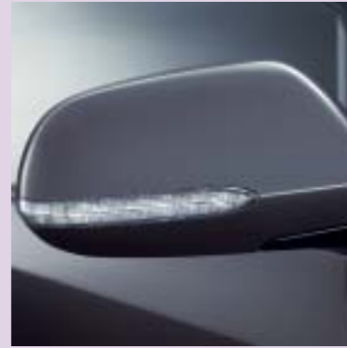
Indicator repeater - Mounting the indicator repeaters in the door mirrors makes them easier to see. Which is good news for everyone on the road (Only available on Executive and Type-S grades).
