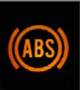
ABS and DSC The Anti-lock Braking System (ABS) with Electronic Brake-force Distribution (EBD) adjusts the braking force to suit the handling, while Dynamic Stability Control (DSC) responds to swerving tendency and stabilises the vehicle within milliseconds.
