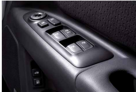
The driver's door console includes switches for the electric mirrors and windows.
