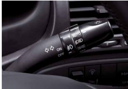
The headlights are controlled by an auto-light control so they can automatically turn on at dusk and off at dawn.
