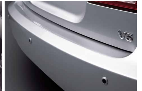
The reversing distance sensors serve as a useful parking aid (on higher grades).
