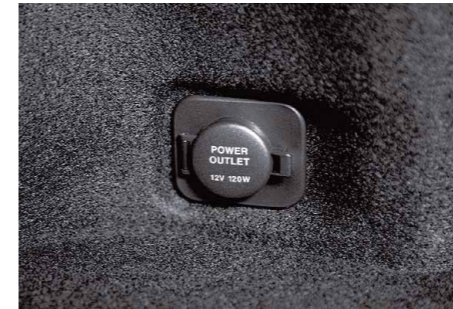
The luggage space comes with a useful auxiliary DC power outlet that comes in very handy for electronic devices such as portable refrigerators.
