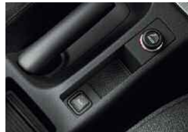
AUX-IN socket in front centre compartment (standard on Sport and S line)
