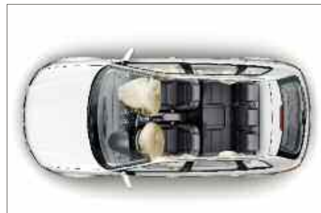
Driver, passenger and side airbag system (rear side airbags optional)
