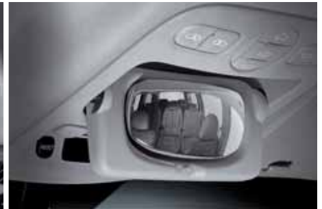
The conversation mirror allows the driver to see everything that's going on in the back at a glance.
