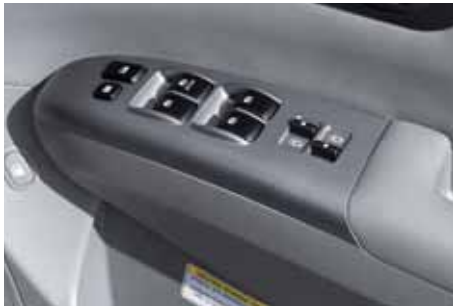
The driver's control panel includes electric window switches as well as the central door locking switch and electric window lock.
