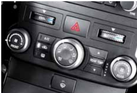
Manual tri-zone air conditioning.
