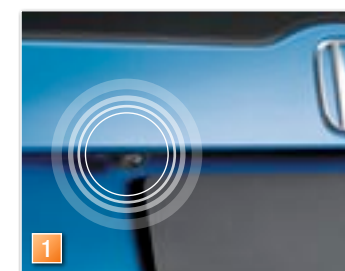
1. PARKING AID CAMERA When reversing, this camera lets you see what's behind your car on the Hard Disk Drive Navigation System's display.
