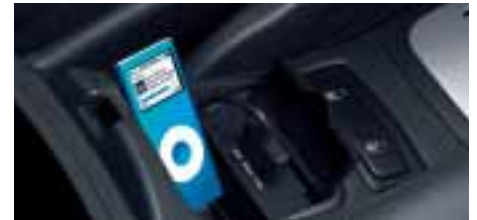
The AUX/USB port allows you to connect to external multimedia sources such as MP3 players and iPods®. From the XS version upwards, the official iPod® cable is included.
