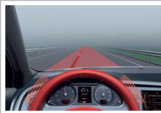
Audi lane assist – steering wheel vibration
