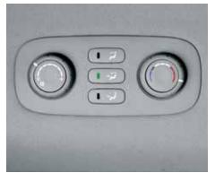
For the comfort of second-row passengers, there are separate temperature controls and fan settings in the rear of the cabin.
