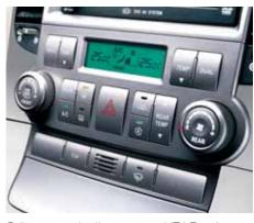
Fully automatic climate control (Tri-Zone). Standard on 2 and 3 models.
