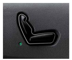
The driver's seat features a 6-way electrical adjustment function so you can find your optimal driving position.
