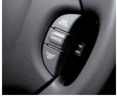
Cruise control helps the driver to maintain a constant speed, particularly useful on long trips and helps ensure speed limits are observed.
