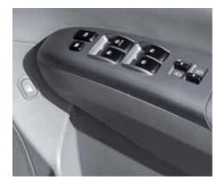
The driver's control panel includes electric window switches as well as the central door locking switch.
