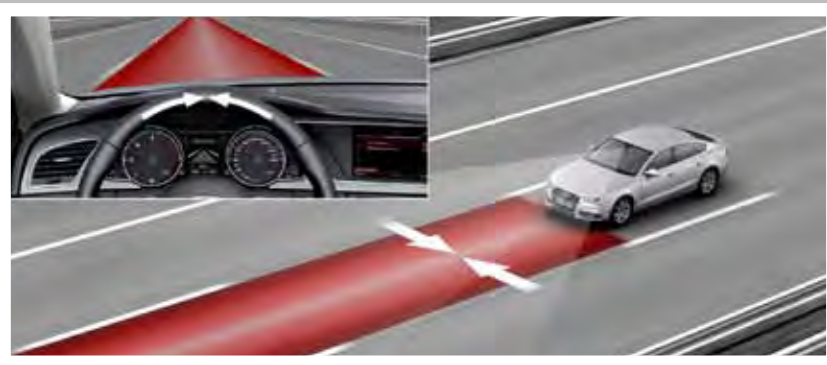
Audi active lane assist (setting 1: early steering intervention)
