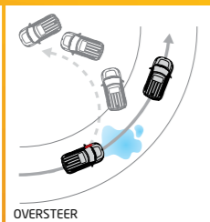
Electronic Stability Control (ESC), fitted as standard to every Soul, improves stability (correcting understeer and oversteer) in extreme driving conditions.
