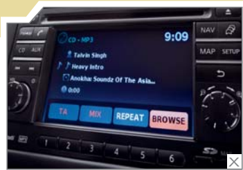
CD RADIO WITH TA. The CD player plays ordinary music CDs, of course, and your own recorded CD-ROMs with MP3, WMA and WAV files. Nissan Connect receives Traffic Management Control (TMC) messages that help you avoid traffic delays.
