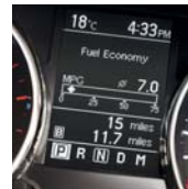
New combimeter: Ultra-clear, chrome-trimmed dials and a large, central LCD display for improved readability.
