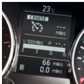
New combimeter: Ultra-clear, chrome-trimmed dials and a large, central LCD display for improved readability.
