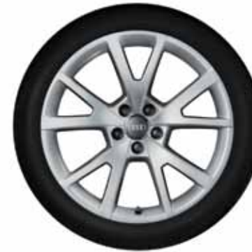
18" x 7.5J '5-spoke V' design alloy wheel with tyre, Part number: 4G0073017B8Z8 (left), 4G0073018B8Z8 (right)
