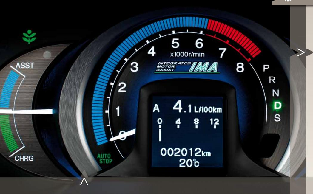
The Insight uses Integrated Motor Assist (IMA), Honda's unique hybrid technology that combines an electric motor with a conventional petrol engine and controls how they work together. Not only does IMA greatly improve fuel economy but it also brings down CO<sub>2</sub> emissions to 96g/km.
