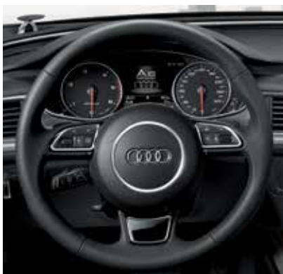
3-spoke leather trimmed multi-function steering wheel with paddles
