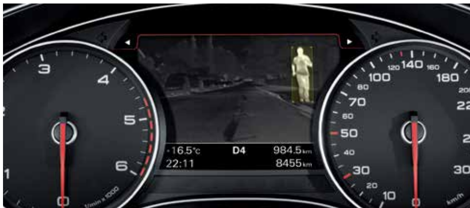
Night vision assistant with pedestrian detection
