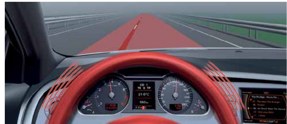
Audi lane assist – steering wheel vibration
