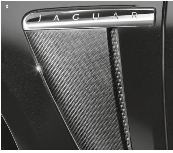
1. CARBON FIBRE MIRROR COVERS 2. CHROME MIRROR COVERS 3. CARBON FIBRE SIDE POWER VENTS
