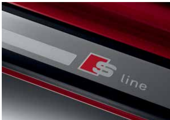
Door sill trims with aluminium inlays and S line lettering
