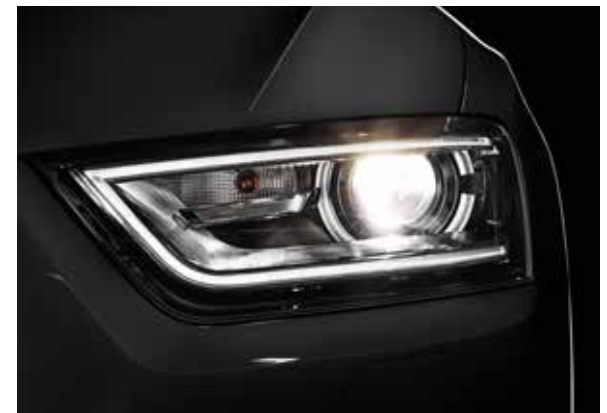
Xenon Plus headlights with LED daytime-running lights strip
