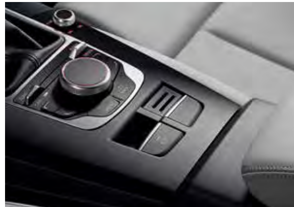
Electromechanical parking brake and MMI control panel
