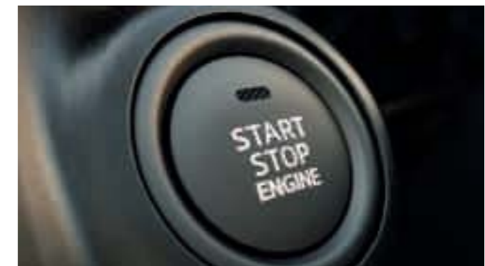
Engine start / stop button Allows you to conveniently start or stop the engine without having to insert the key.
