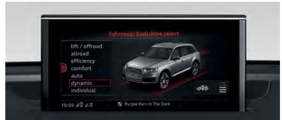
Audi Drive Select – image features modes that are available with optional Adaptive air suspension
