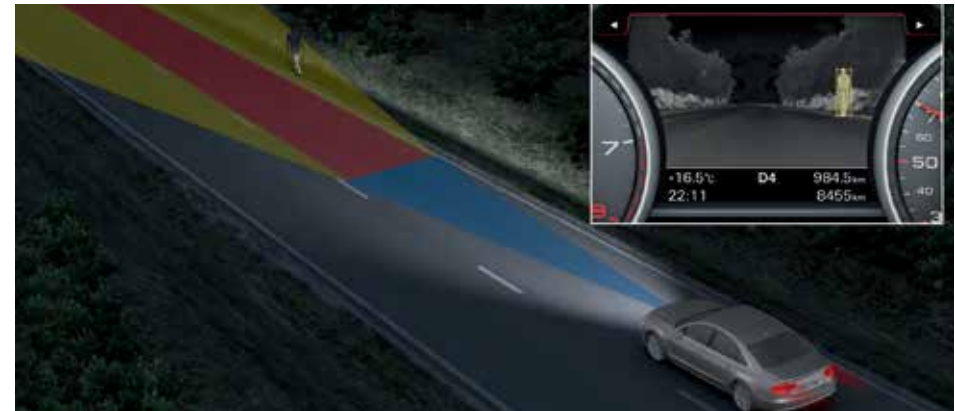
Night vision assistant with pedestrian and animal detection
