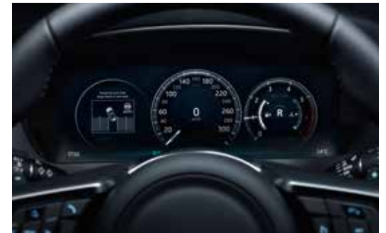
12.3 inch Instrument Panel Display with virtual dials
