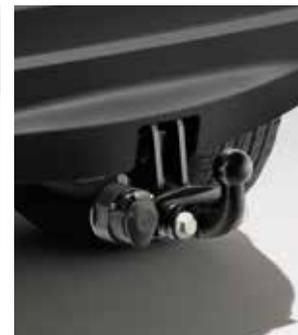
**Towing System – Fixed Height Flanged Tow Bar\*\***
