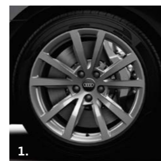
Main images. A8 in Vesuvius grey, metallic paint. 1. 18" x 8.0J '5-V-spoke' design forged alloy wheels. 2. LED rear lights. 3. Twin-spoke leather multi-function steering wheel with shift paddles. 4. Comfort front seats in Valcona leather.
