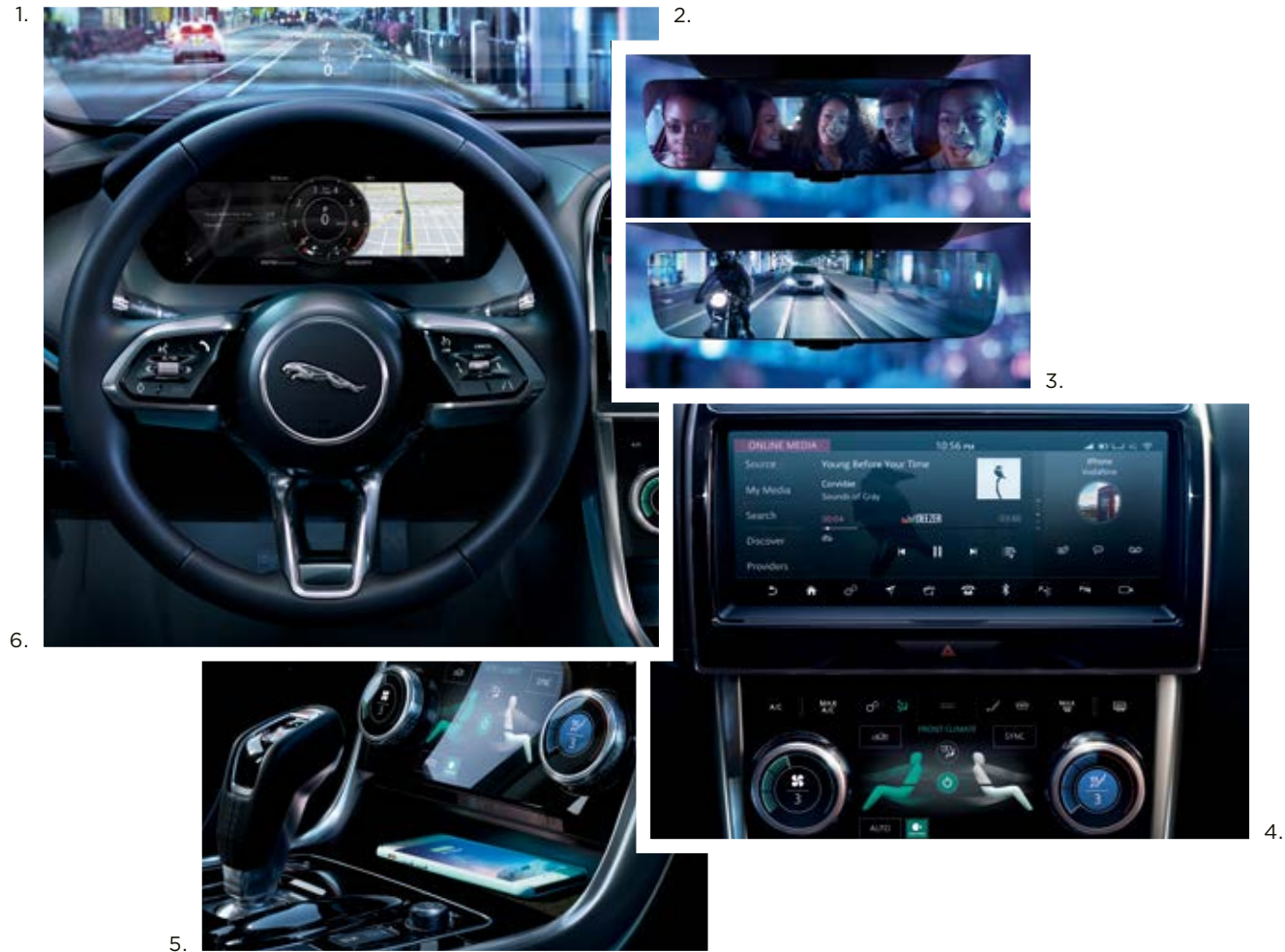
(1) Head-up Display (2) Solar attenuating windscreen (3) ClearSight interior rear view mirror* (4) Touch Pro Duo (5) Wireless device charging (6) Interactive Driver Display.
