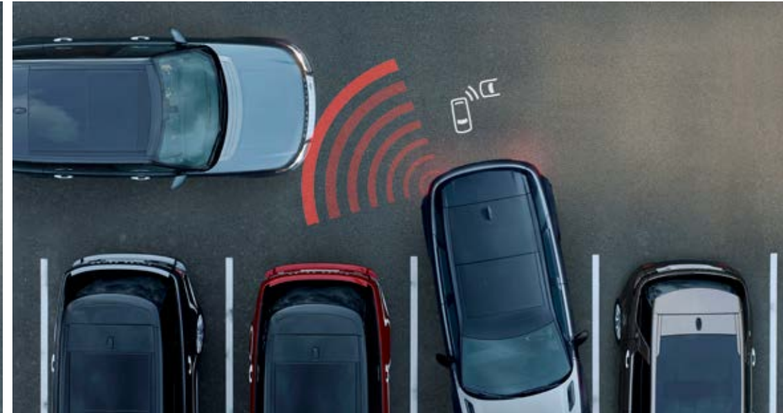
Rear Traffic Monitor
