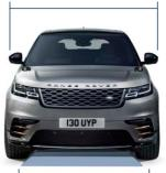
Front wheel track 1,644mm (Air), 1,640mm (Coil)†
