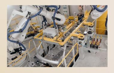
Smooth laser-welded interface rather than a traditional roof finisher provides a seamless finish in support of Land Rover's design philosophy.
