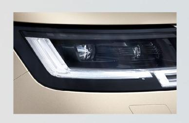
Digital LED headlights with industry leading microprocessor and 1.2 million micromirrors, can focus on 16 objects simultaneously and blank out reflections.
