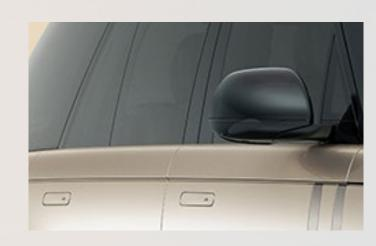
The rounded edge of the door meets the glass in a simple, clean finish thanks to a specially engineered hidden waist finisher.
