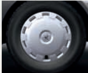
14-inch steel wheels with flush covers and 175/70 R 14 tyres.
