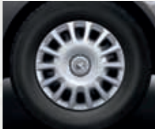
14-inch steel wheels with flush covers and 185/70 R 14 tyres.
