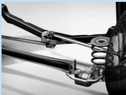
Watt's link improves handling and ride comfort.
