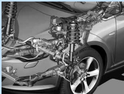
MacPherson strut front suspension.
