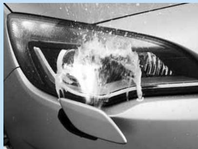
High-pressure headlight washers.
