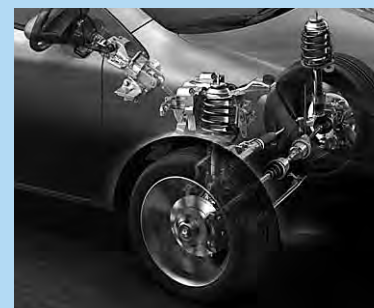
MacPherson strut front suspension.
