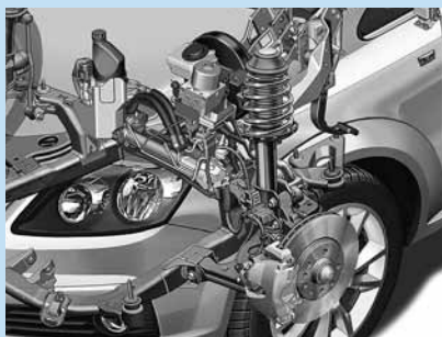
MacPherson strut front suspension.
