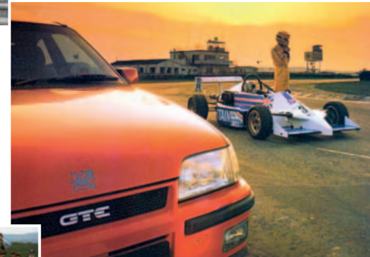
1984 – The MkII Astra introduced class-leading aerodynamic styling that still looks good today. The Formula Vauxhall Lotus ran a modified version of the Astra GTE's 2.0i 16v engine.
